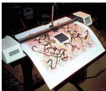
Roman Verostko, multi-pen plotter showing Chinese brush mounted on drawing arm executing a brush stroke. 1987, Hi-DMP multi-pen plotter (pen stalls removed for paint brush routine). Courtesy of the artist.
